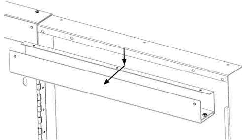
**Step 3:** Remove two nuts from inner cassette, lift of plate, and remove and replace inner gasket.
