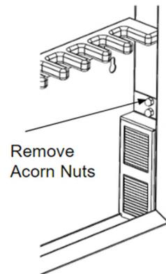
**Step 3:** Remove and replace HEPA filter.
