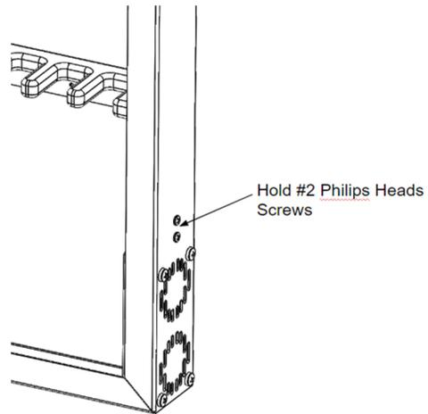
**Step 2:** Remove acorn nuts with nut driver
