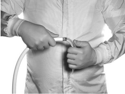
FIGURE 4. REMOVE THE DETACHABLE TIP WITH A PEELING MOTION
