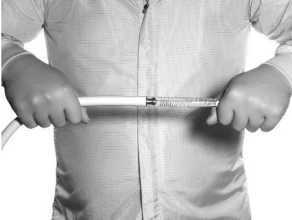
FIGURE 5. INCORRECT REMOVAL OF DETACHABLE TIP
