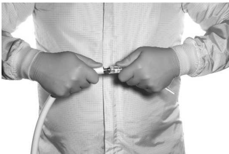
FIGURE 3. ATTACHMENT OF THE DETACHABLE TIP TO THE FIBER OPTIC CABLE.
